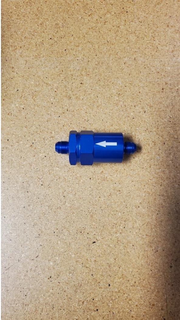
On the new install, the AN fittings are integrated directly into the FILTER mechanism. Some of the filters have arrows indicating flow direction. If they do not, the side with the double nut is the OUTPUT side.
